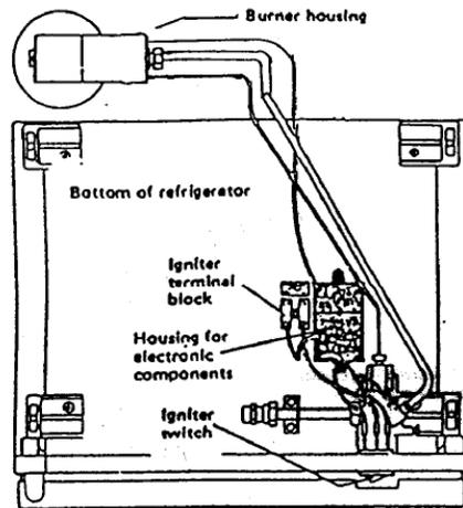
**Fig. 11** View of bottom of refrigerator showing electronic igniter layout.
