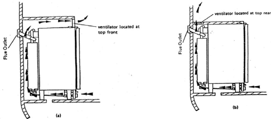
Arrows indicate air-flow to ventilate cooling unit at rear
